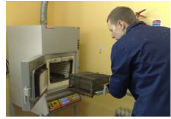
Figure 5 - Conditioning Sample Bitumen Content for Cold Mixes, Macadam's etc.
