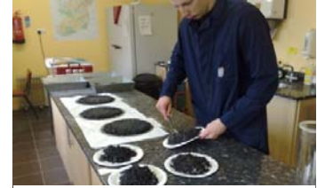
Figure 3 - Site Samples These are mix designs for Cold Mixes
